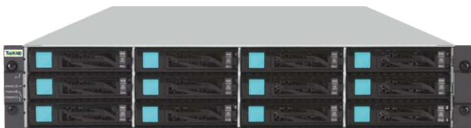
TopRAID M100/M300 Series with 24 x 3.5 LFF drive bays
